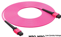
MPO-MPO Low Smoke Halogen 2000-20000 Multimode 10 Gigabit 12 ports OM4 Insertion loss: 0.25dB Return loss: >20dB
